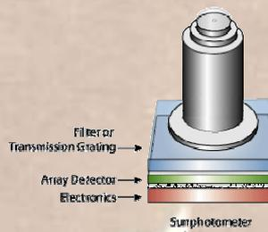
Two prototypes of the Advanced Sunphotometer have been assembled. The reflecting optic is a cone that is 25 mm high with entrance and exit apertures of 1 mm and 12.5 mm respectively. The first prototype (see Figure at right) used a Vitana PixeLink PL A653 array with 8 bit resolution.
