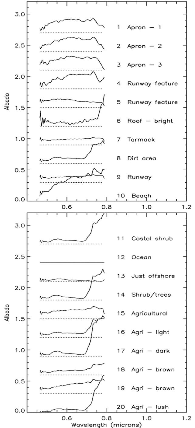
Fig. 5 - Surface albedo spectra derived from DASI measurements for each of the designated regions of Fig. 1. The dotted lines indicate the albedo scale origin for each region. Identification was aided by color aerial photographs of the scene. Regions 11, 14, 16, 17, and 20 reveal the vegetation red-edge feature caused by chlorophyll. The spectra of regions 6 and 10 are badly distorted due to detection saturation.
