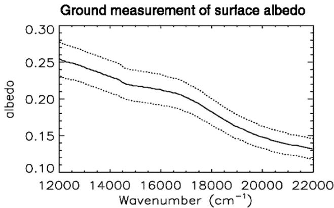
Fig. 3 - Results of surface albedo measurement of designated region 1 in Fig. 1. The standard measurement error (dotted curves) is shown about the mean value (solid curve).
