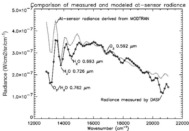
Fig. 4 - DASI derived spectrum corresponding to region 1 of Fig. 1 (solid curve with symbols) together with a modeled spectrum derived from MODTRAN and the surface albedo measurement of Fig. 3 (dashed line).
