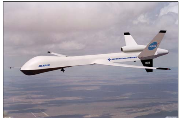
Figure 6. GA-ASI ALTAIR® UAV. The ALTAIR® is an offshoot of the Predator UAV and allows larger payload capabilities, higher altitude, longer range and extended mission duration.
