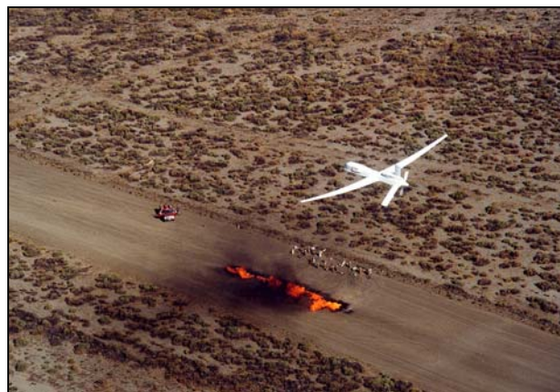
Figure 2. The ALTUS II® UAV containing the NASA-Ames AIRDAS imaging payload on low pass prior to landing. Flames and smoke from the controlled burn, ignited earlier, can be seen below the aircraft.
